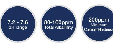
2. A pH of less than 7.0 should be especially avoided as it can cause the liner to form wrinkles, with greater probability if the water hasn't been stabilized with cyanuric acid and the chlorine is maintained at or above superchlorination levels for extended periods. For this reason, it is recommended that all vinyl lined swimming pools be routinely stabilized with cyanuric acid and that a minimum of 50 ppm be maintained.
